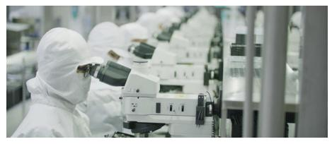
The testing process is long, complex, and manually intensive. There are 100,000 sliders in every 200mm wafer that need to be checked. The Normandale factory takes millions of microscope pictures every day, generating 10TB of data that must be sifted to detect potential production defects before wafers are assembled into drives.
